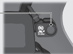
ABS function on both wheels is on.
