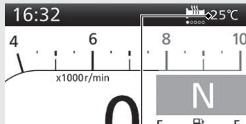
Air temperature gauge
