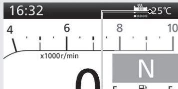
Air temperature gauge
