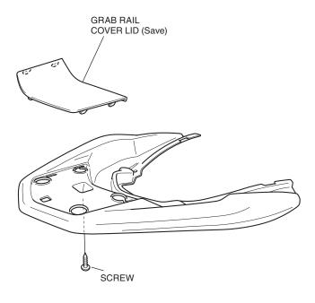
4. Install the carrier base as shown.
