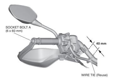
7. <DCT type right side only> Install the cable clip to the right knuckle guard stay as shown.
