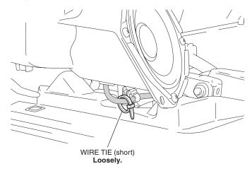
41. Route and secure the CB antenna code as shown.
