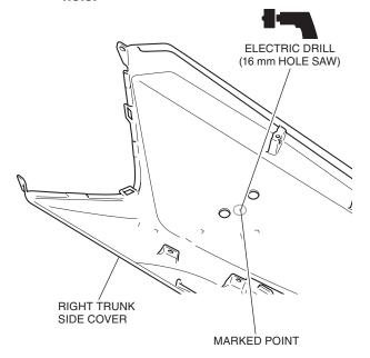
35. Clean the surface of the area shown using an isopropyl alcohol.
