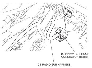
57. Secure the CB radio sub harness with the wire tie as shown.
