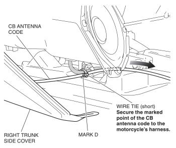
42. Secure the CB antenna code with the wire tie as shown.
