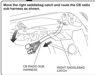
30. Connect the CB radio sub harness as shown.
