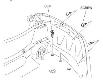
11. Remove the parts as shown.
