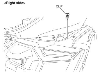
16. Remove the rear fender as shown.
