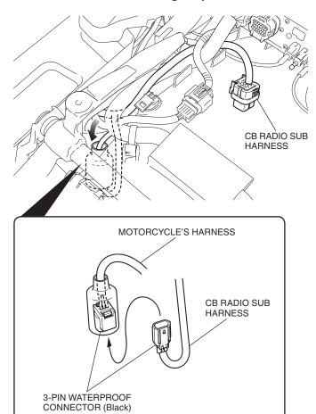
55. Remove the dummy connector as shown.
