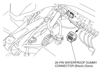
56. Connect the CB radio sub harness as shown.
