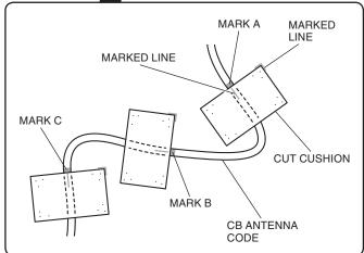
40. Loosely install the wire tie as shown.
