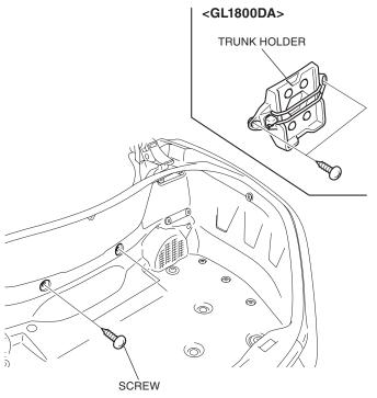
9. Remove the front trunk lower panel as shown.
