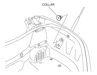
49. Install the CB antenna stay as shown.
