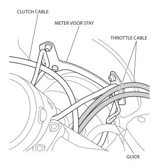
8. Move the handlebar right and left, and check that this accessory is not interfere with the motorcycle parts.
