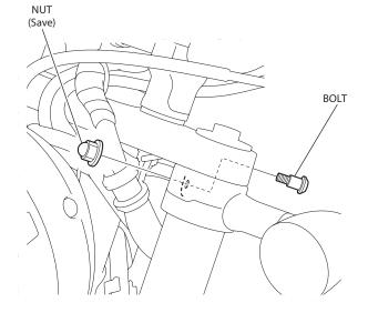
3. Loosely install the meter visor stay as shown.
