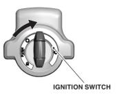
2. Push the SET button 3 times within 10 seconds and turn the ignition switch to the OFF. The buzzer sounds for 1 time.
