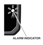
The alarm indicator flashes while the alarm system activated.
