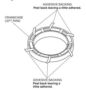
3. Attach the crankcase left ring as shown.
