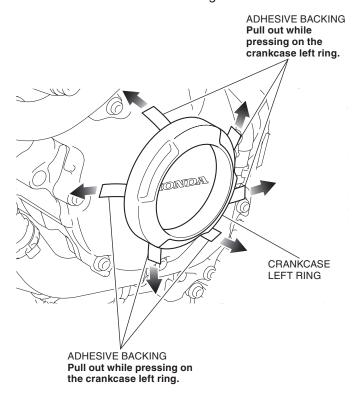
5. Apply adequate pressure to crankcase left ring.
