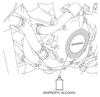
2. Peel off the adhesive backing on the crankcase left ring as shown.
