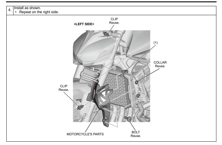
Install the motorcycle's parts in the reverse order of removal.
