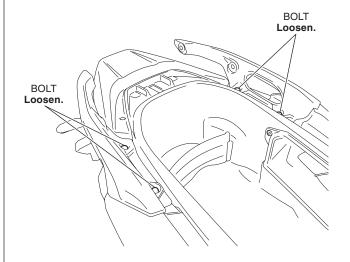
4. Loosely install the rear carrier as shown.
